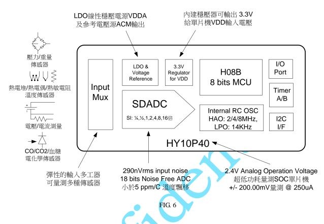
HY10P-series 8-bit high-performance OTP MCU provided by HYCON is as shown in FIG. 5. The MCU not only includes the over sampling sigma delta analog-to-digital converter, but also can significantly simplify the peripheral circuit of the application; the chip is actually a MCU with high-performance specification and high integration:
