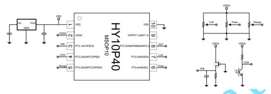
FIG. 4 Application circuit of HY10P40 PIR detector
