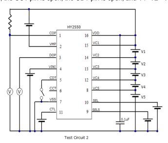
7.3.1 Overcharge Detection Voltage (VCUn) · Overcharge Release Voltage (VCRn)
