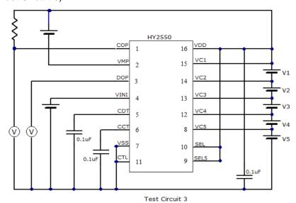
Confirm that the COP pin and DOP pin are "L" when VVMP =VDD, VINI =VSS, and V1=V2=V3 =V4= V5=3.5 V (this status is referred to as the initial status.
